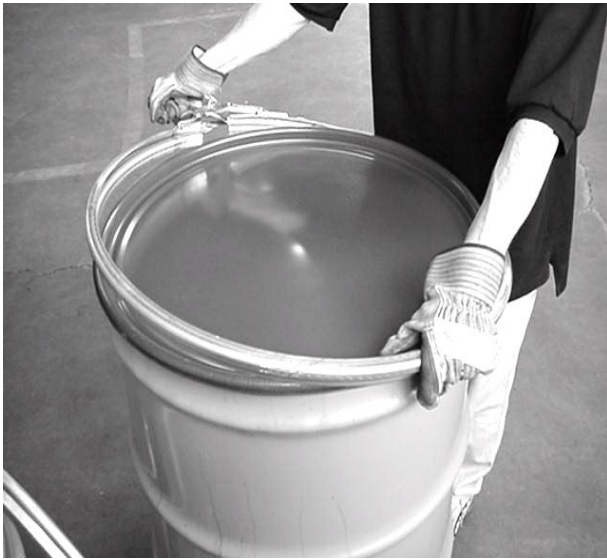
Expanded ring being placed on Drum
